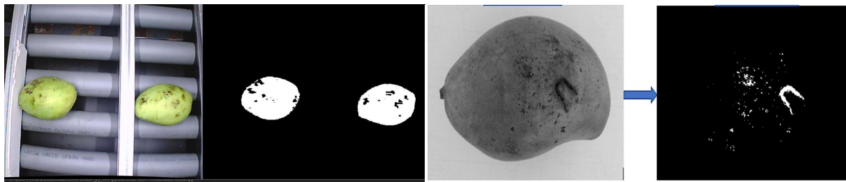
Figure 3.14. Convert RGB color image to gray image and Convert gray image to binary
